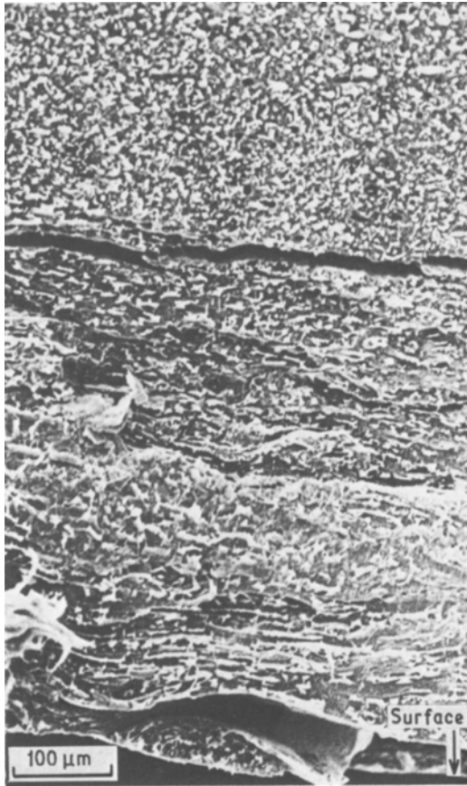
Figure 4 Scanning electron micrograph of the fracture surface of the test bar moulded at a high mould temperature (60° C) and low injection pressure (45 MPa) (lower overall orientation). Close to the surface the polyethylene “fibres” are ribbon-shaped, while at about 0.4 to 0.5 mm from the surface they change to a more circular cross-sectional area.
